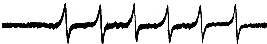
FIG. 23.16. Hyperfine structure of the ^{55}\text{Mn} ( I = \frac{5}{2} ) nucleus in the electron spin resonance spectrum of a \text{Mn}^{++} ion ( S = \frac{5}{2} , transition S_z = \frac{1}{2} \leftrightarrow -\frac{1}{2} ). The resonance condition is h\nu = g\beta(B_0 + B_n) , where B_n is the magnetic field due to the nucleus. In first approximation B_n is proportional to the nuclear magnetic quantum number I_z ; this gives a pattern of 2I + 1 = 6 lines, equally spaced and of equal intensity, since all nuclear orientations are equally probable at the temperature of the observation. The line shape is the derivative of the absorption curve; it is obtained by a sinusoidal modulation of B_0 with amplitude small compared with the line width. This gives a corresponding modulation of the signal (measured by a phase sensitive detector) whose amplitude is proportional to the slope of the absorption curve.
